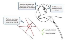
Position the SilhouetteStar facing the wound so that the laser lines cross near the center of the wound to form a star shape. The laser lines do not need to cross in a perfect star shape, but all the crossing points should be within the wound. One of the laser lines should cross the deepest part of the wound. For very large wounds, see the instructions in "Taking a Multiple Image Measurement" on page 11.
