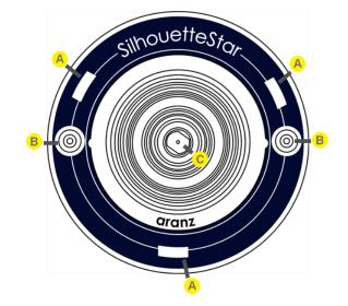
The location of SilhouetteStar's laser lights, LEDs, and camera lens are shown below:
