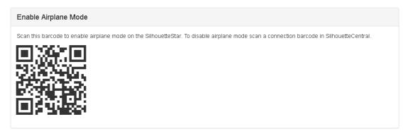
Once the device is in airplane mode it will remain in airplane mode until a connection barcode is scanned to attempt a Wi-Fi connection to SilhouetteCentral.
