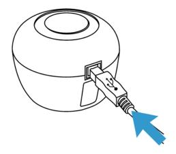
Insert the flat end of a SilhouetteStar USB cable into one of the USB 2.0 or 3.0 ports on your computer:
