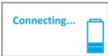
The device is attempting to connect to the specified wireless network. If the connection fails, ensure you are in range of the correct Wi-Fi network. If the connection is still not successful, contact your system administrator. The Wi-Fi icon is replaced by a USB icon when the device is connecting to SilhouetteConnect via a USB cable.
