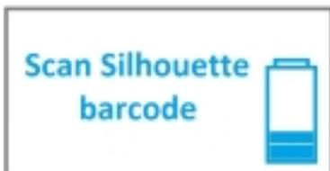
The device is fully powered up and is waiting for the user to scan a QR code, which enables it to connect to the wireless network or it is waiting for a user to log in to SilhouetteConnect on a computer it is connected to via a USB cable.
