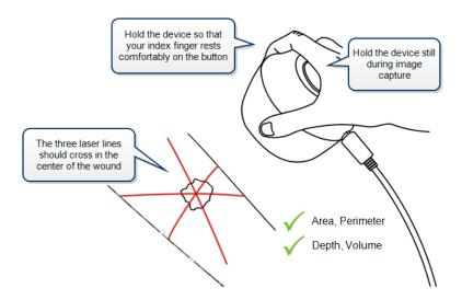
Position the SilhouetteStar device facing the wound so that the laser lines cross inside the wound to form a star shape. The laser lines do not need to cross in a perfect star shape.
