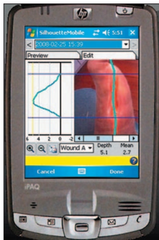
Figure 6. SilhouetteMobile displaying depth assessment and profile
