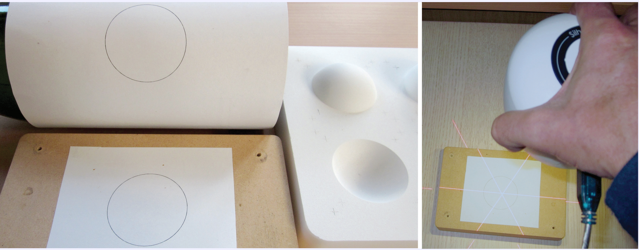
Figure 1: Left photograph shows the four wound models - disk on a cylinder (top left), disk on a flat sheet (bottom left) and convex and concave sections of a hemisphere (top and bottom right respectively). The right photograph shows the device capturing data from the flat model.
