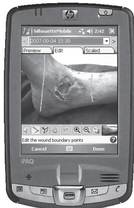
Figure 1: The ARANZ Medical SilhouetteMobile : Capturing the image for surface area measurement (top) and user-drawn wound boundary (bottom). Note the stylus in the top image (held in the clinician's right hand), which is used, for drawing the wound boundary on the PDA touch-screen.
