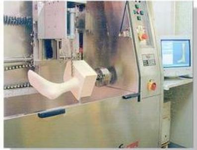
Figure 1: The process of scanning a plaster cast
