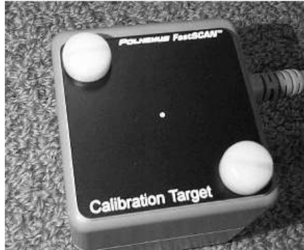
Figure 29: The Transmitter with the Calibration Target attached.
