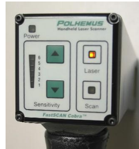
(d) Wand control panel showing Laser-On indicator light (top-right LED)
