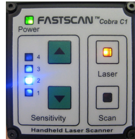
(b) Wand control panel showing Laser-On indicator light (top-right LED)
