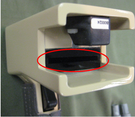
(a) Close-up of the laser aperture (circled), and two-position trigger switch (bottom).
