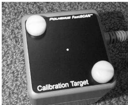
Figure 28: The Transmitter with the Calibration Target attached.
