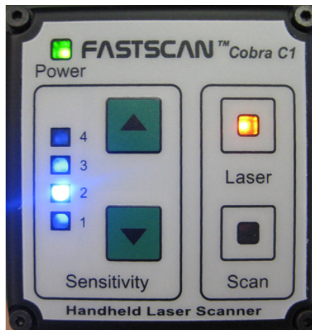
Figure 8: The Wand control panel with the power and Laser lights illuminated.
